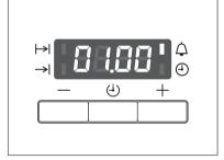
When the time has elapsed, the function indicator flashes and an audible signal sounds for 2 minutes. The signal can be stopped by pressing any button.
